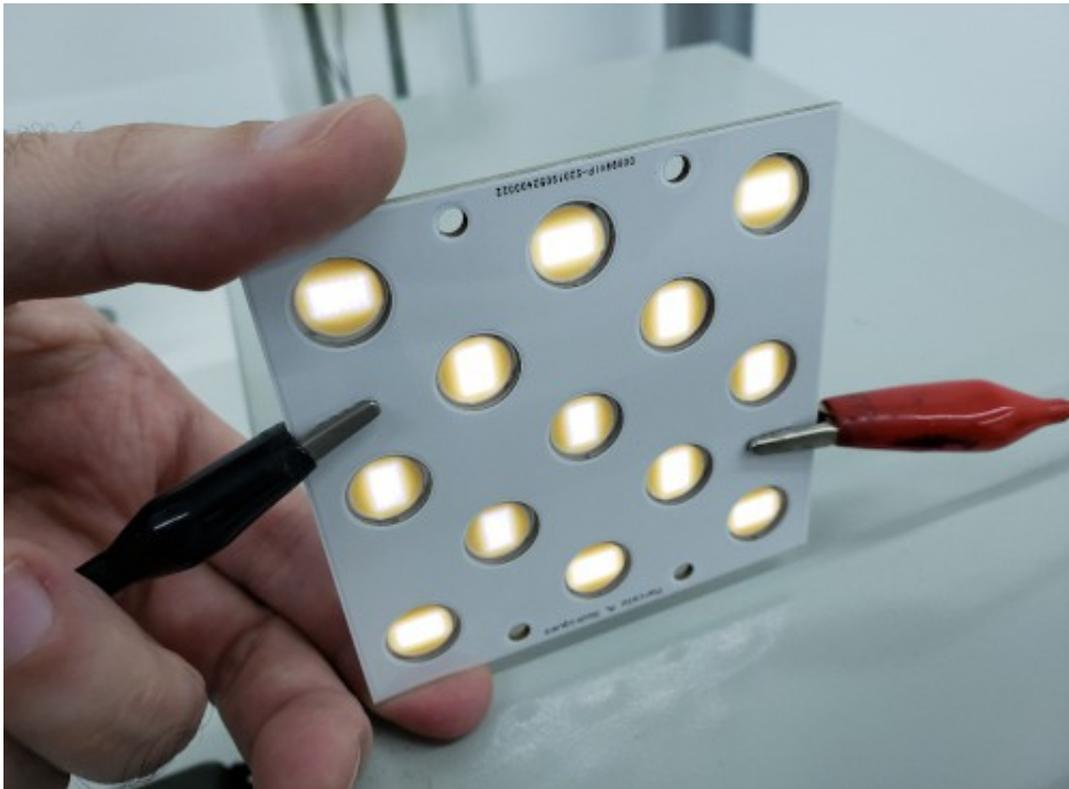
**Figure 5.7:** Lamp fabricated with white LEDs Yuji International® model YJ-VTC-135L-G01.
