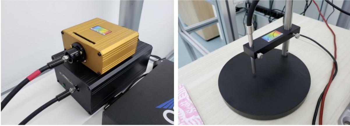
**Figure 5.11:** Spectrometer setup used for thickness measurement
