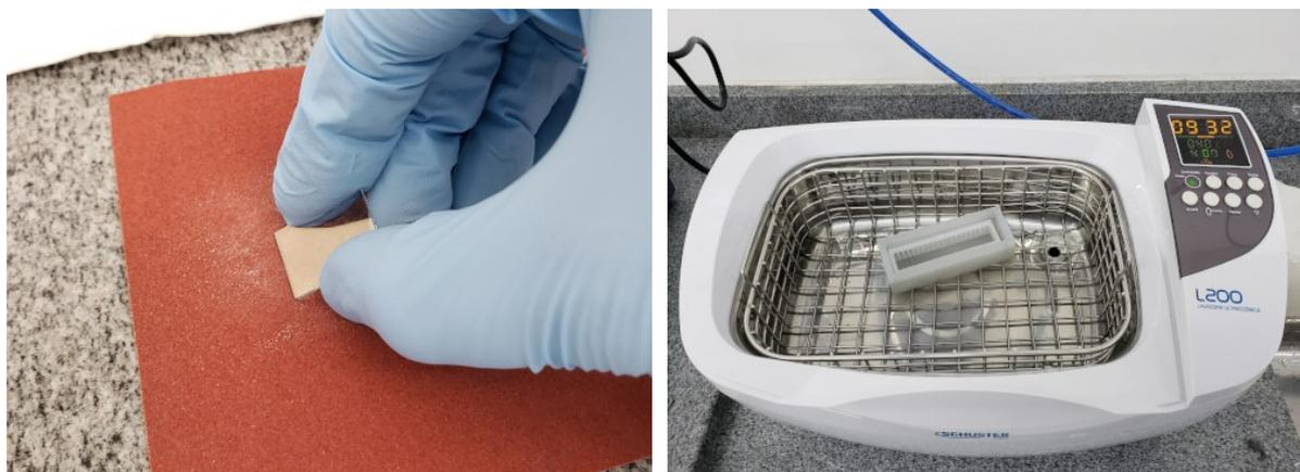
**Figure 5.4:** Substrate preparation and cleaning.
