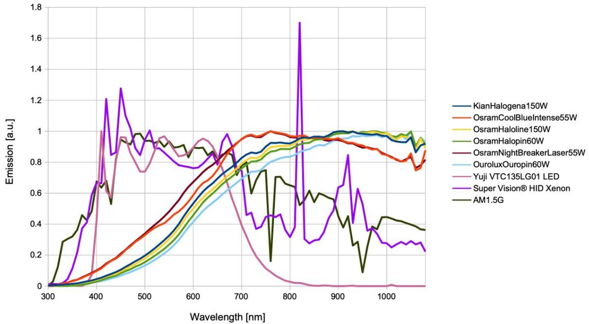
**Figure 5.8:** Lamps spectra versus AM 1.5 spectrum.
